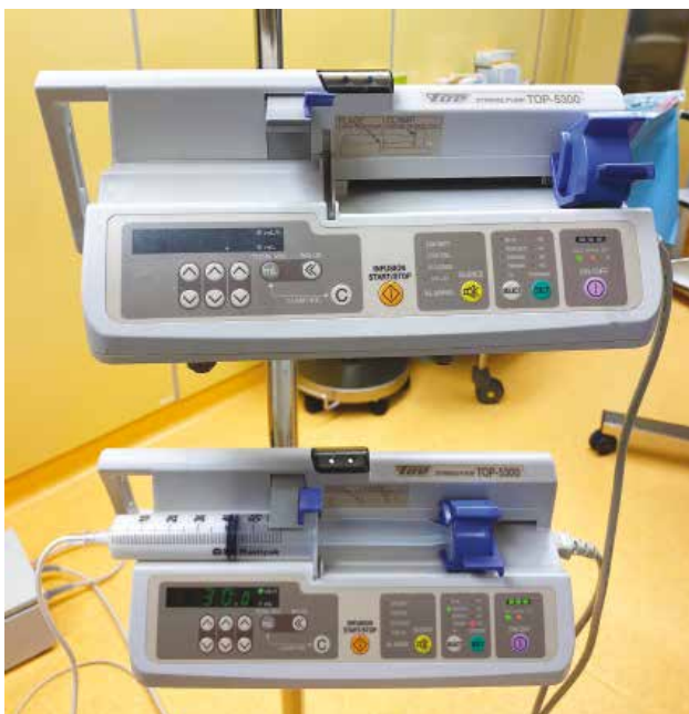
FIG. 3 Programmable syringe pump for anesthesia.
